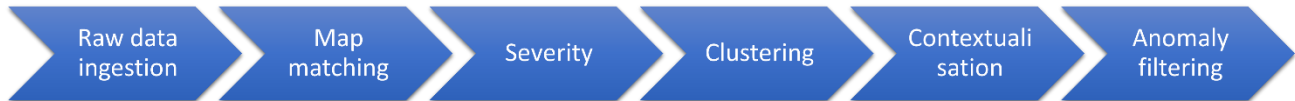
Figure 3 – Data processing pipeline. The map-matching procedure allows to convert raw GPS data into positions on the road network. The clustering algorithm itself is the core of our approach to predict future accident locations. The contextualisation step enables us to reject anomalies in the data.
